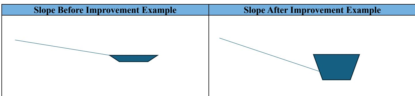
As illustrated above; by deepening the outlet, a drainage district effectively increases the available "fall" or slope for a private tile system. This allows a landowner to drain otherwise flat or depressional areas and enables them to use smaller, less expensive tile to achieve the same drainage capacity, a direct economic benefit.
